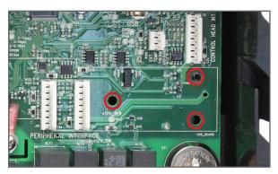
5. Attach the 5 Port Communication Hub to the control board. Line up the connector on the hub with the header on the control board, and the standoffs with the standoff holes.
