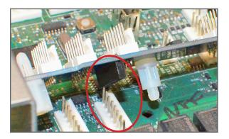
6. Press on the top of each of the standoffs on the 5 Port Communication Hub till they click into place.
