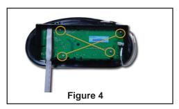
**Step 4.** Install the control head assembly to the control box.
